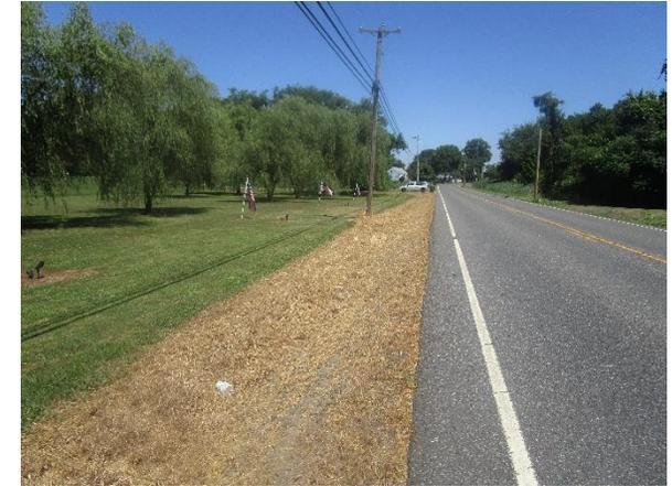
The trench stretching along the east side of the road can be converted into a rain garden to allow stormwater runoff from the road to infiltrate more efficiently. Creating a rain garden will also benefit wildlife by creating habitat. A preliminary soil assessment suggests that more soil testing would be required before determining the soil's suitability for green infrastructure.
