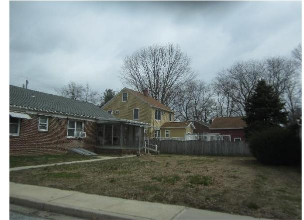
Bioretention systems can be installed in the turfgrass on both sides of building to capture, treat, and infiltrate stormwater runoff from the roof. A preliminary soil assessment suggests that more soil testing would be required before determining the soil's suitability for green infrastructure.
